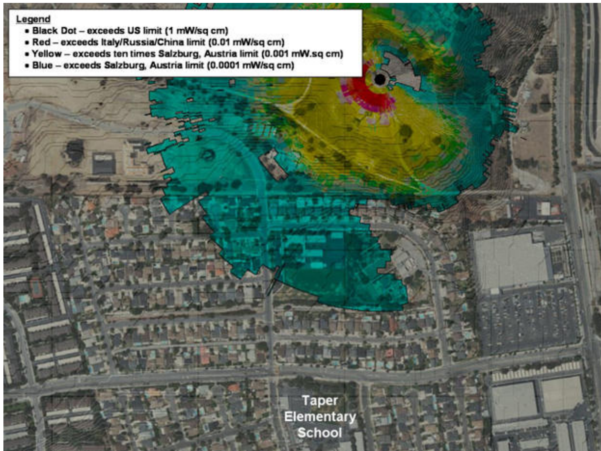
Figure 4: Exposure contours if the tower was located within the uninhabited San Pedro Fuel Depot instead of within the Westmont neighborhood. Note that no residences fall within the red or yellow contours (greater than 0.001 mW/cm 2 ) and only a small portion of the neighborhood falls within the blue contour (0.0001 mW/cm 2 ). Compare to Figure 2.
