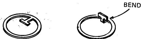
Figure 2-4. Indicator Cable Mounting Details
